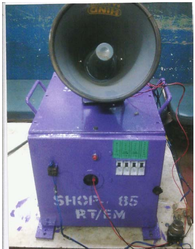
Sri S.Rajendran, Tech, Shop-85, has made a siren to alert the nearby staff while shunting the coaches. The siren can be operated manually and also by giving a missed call to a phone number attached to the siren. Once it starts, the duration can be set in minutes from one minute to one hour. Now, while pushing the coach on reverse, the loco pilot can give a missed call from his seat and the siren will start alerting the passerby. He is on the job to make a device for un manned level crossings to sense the incoming train and give siren automatically.
